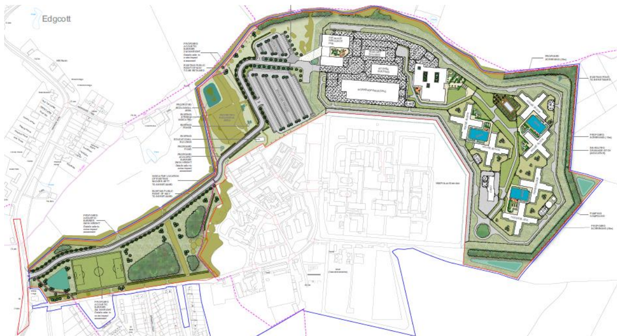
Figure 1 Schematic of proposed plan showing road and access point to the main construction area and final site
